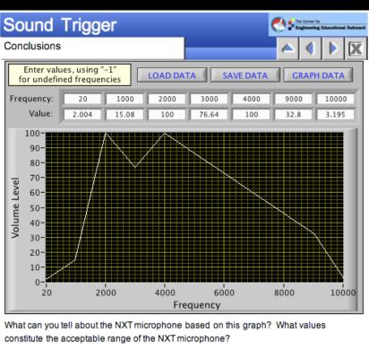
the NXT microphone picks up some values better than others. For example, the amplitude at 3,000 was a lot lower than the surrounding values. From 20 to 10,000, the NXT picks up a range of values.
