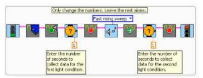
The code above will allow the NXT to collect data with the light sensor. Change the times the sensor is collecting data to match the graph to the right. The light sensor will click when it is collecting data and then beep to tell you to switch lighting conditions. Collect data and try to match the graph by clicking the arrow button and running the program on the NXT.
